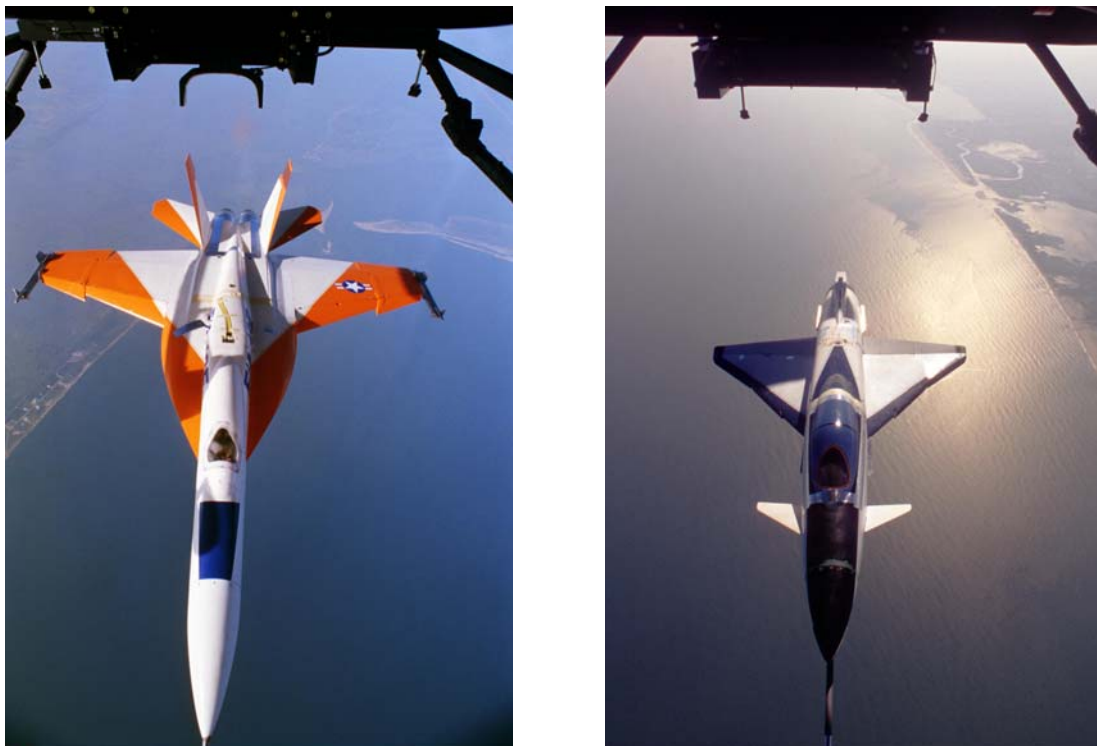
Figure 2: F-18 (l) and X-31 (r) Drop Models just after release from helicopter
