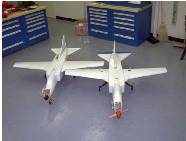
Figure 8: “Very Small UAV” weighing approximately 15 lbs.
