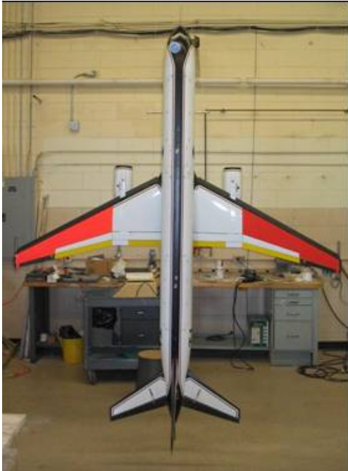
Figure 5: Inertial Testing of a Dynamically Scaled Model
